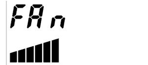
During fan speed modification, if no key is pressed for about 10 seconds, normal operation will resume, preserving any modifications that have been made.
