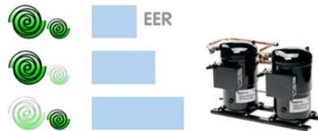
THE SEQUENTIAL DEACTIVATION OF THE COMPRESSORS INCREASES EFFICIENCY
