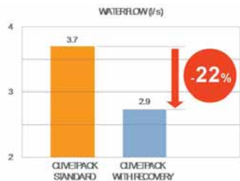
Example for a unit of 16.000 m 3 /h in commercial application in continental climate
