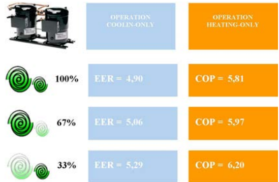
Example referred size 45.2 at conditions:: W35/W7 cooling only, W10/W35 heating only
