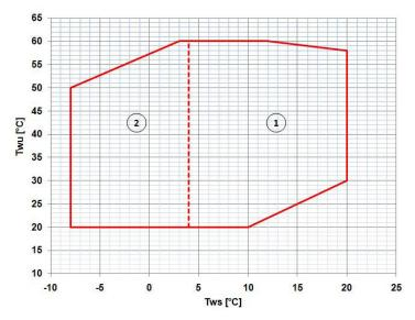
Twu [°C] = Leaving water temperature user side / hot Tws [°C] = Leaving water temperature source side / cold The limits refer to DT=5 °C on both the heating and cooling sides
