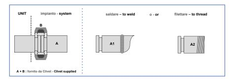
O not weld the system pipe with the Victaulic connection joint attached. The rubber gasket might be irreparably damaged.
