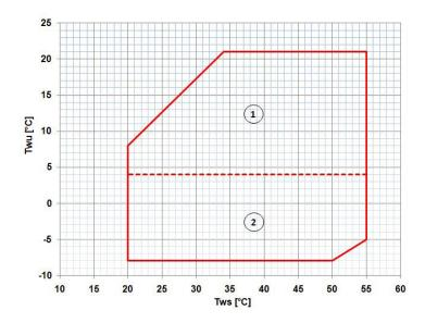
Twu [°C] = Leaving water temperature user side / cold Tws [°C] = Leaving water temperature source side / hot The limits refer to DT=5 °C on both the heating and cooling sides
