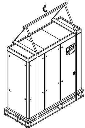
Ensure that the unit is stable and balanced.
