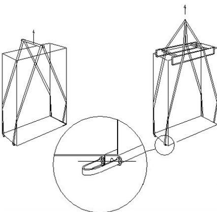
Rigid structure to prevent damage to the structure
