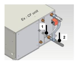
Inlet water temperature probe
