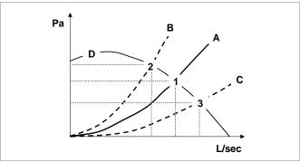
D = unit head-flow rate curve
