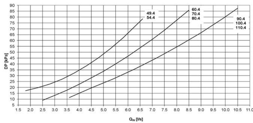
Pressure drops on the water side are calculated considering an average water temperature of 65°C
