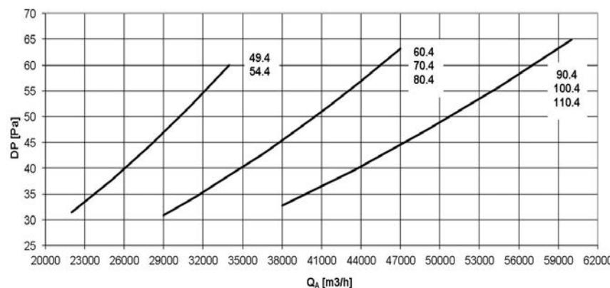
The air side pressure drops are relative to the medium air temperature of 20°C and are to be added to the pressure drops due to ducts, terminal devices and any other component that causes a drop in working discharge head.
