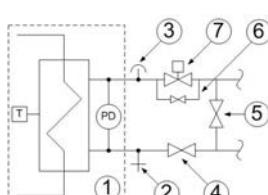
1. plate heat exchanger complete with water side differential pressure switch (to control presence of water flow rate) and a water temperature control probe (to disable the compressors when the water temperature drops below the limit value);
