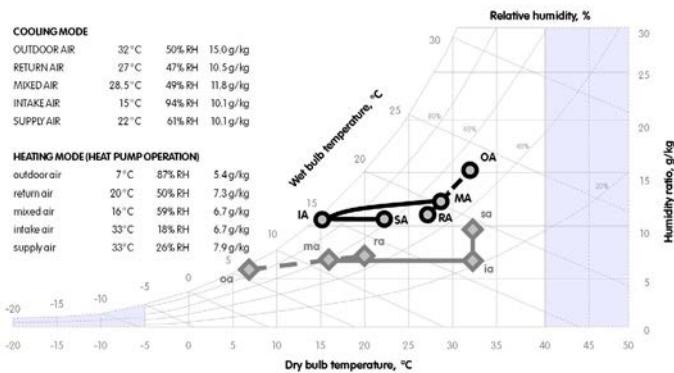
Treatment example at full load for CLIVETPack model CRH-XHE2 49.4 in standard airflow. Outdoor airflow equal to 30% of that treated. Heating carried out with a heat pump. Unit complete with 'post-heating with hot gas' and 'vapour humidifier of 15 kg/h' options.
