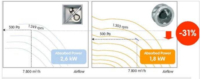
Electrical power absorbed by electric motor, data constructor - Example, referred to flow of 7.800 m<sup>3</sup>/h with 500 Pa external static pressure.
