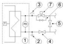
1. plate heat exchanger complete with water side differential pressure switch (to control presence of water flow rate) and a water temperature control probe (to disable the compressors when the water temperature drops below the limit value);
