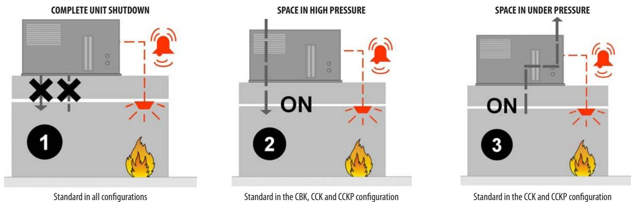
The unit is able to manage the signal coming from a fire detection system or fire control unit installed built-in, activating one of the logics illustrated, which can be set by parameters. In presence of alarm signal, the compressors are always switched off; moreover, the remote ON-OFF is disabled together with the switch on/off control from keypad. The unit is manually reset. Rooftop units cannot be used as fume extractor.
