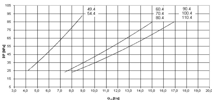
Pressure drops on the water side are calculated considering an average water temperature of 65°C
