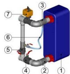
In summer operation, the device, complete with modulating valve, makes it possible to maximize the thermal differential of the water and hence to reduce the water flow rate. In winter operation, modulation of the water flow rate allows the unit to function with the water loop at high temperature. An additional advantage of using this device is the extension of the operating limits of the unit in summer and winter.
