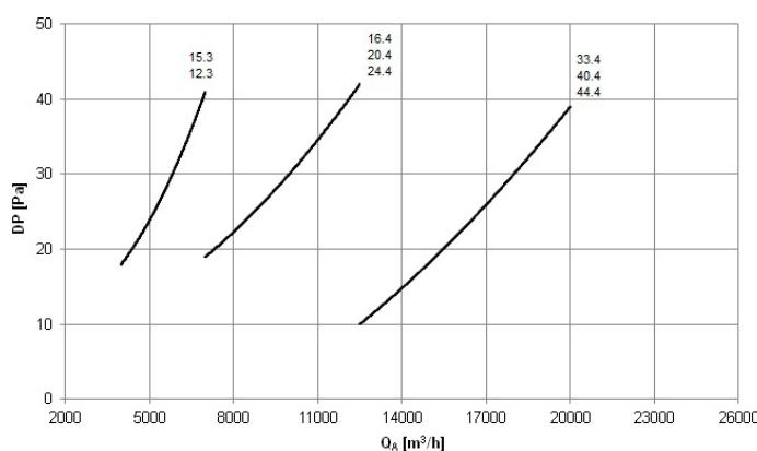
The air side pressure drops are relative to the medium air temperature of 20°C and are to be added to the pressure drops due to ducts, terminal devices and any other component that causes a drop in working discharge head.
