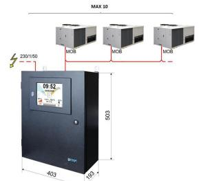
**⚠** The component must be combined with the RS485 serial port option with Modbus protocol built-in of each rooftop.
