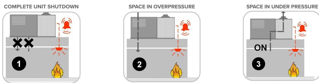
The unit is able to manage the signal coming from a fire detection system activating one of the logics illustrated, which can be set by parameters. In presence of alarm signal, the compressors are always switched off; moreover, the remote ON-OFF is disabled together with the switch on/off control from keypad. The unit is manually reset. Rooftop units cannot be used as fume extractor.
