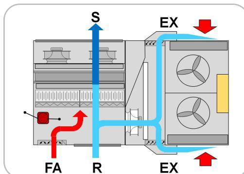
The room pressure control device is fitted as standard in the units with extraction and exhaust (Clivet reference code CCK and CKP)
