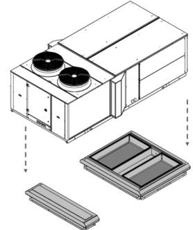
**⚠** If the gas module is selected, provide for an appropriate support structure, the supply air can only be horizontal
