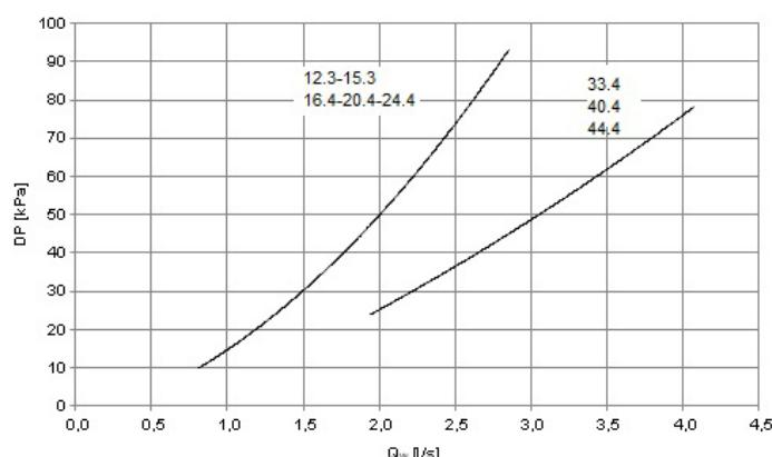
Pressure drops on the water side are calculated considering an average water temperature of 65°C
