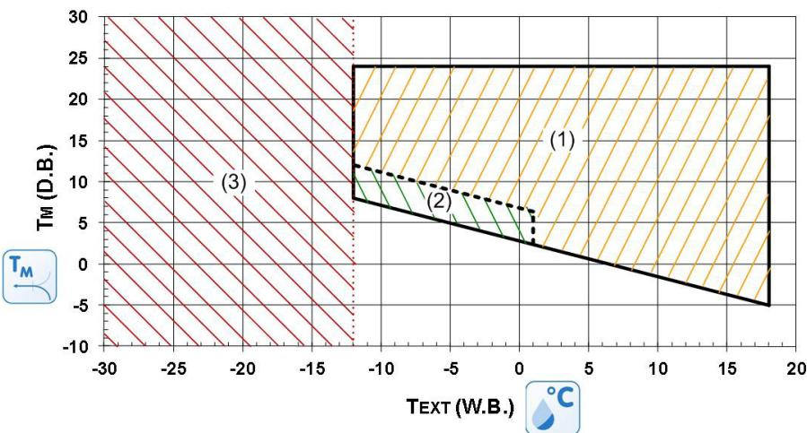
To verify the operating range of the operating units with percentages of fresh air, always calculate the T<sub>m</sub> mixing temperature at the internal heat exchanger input.
