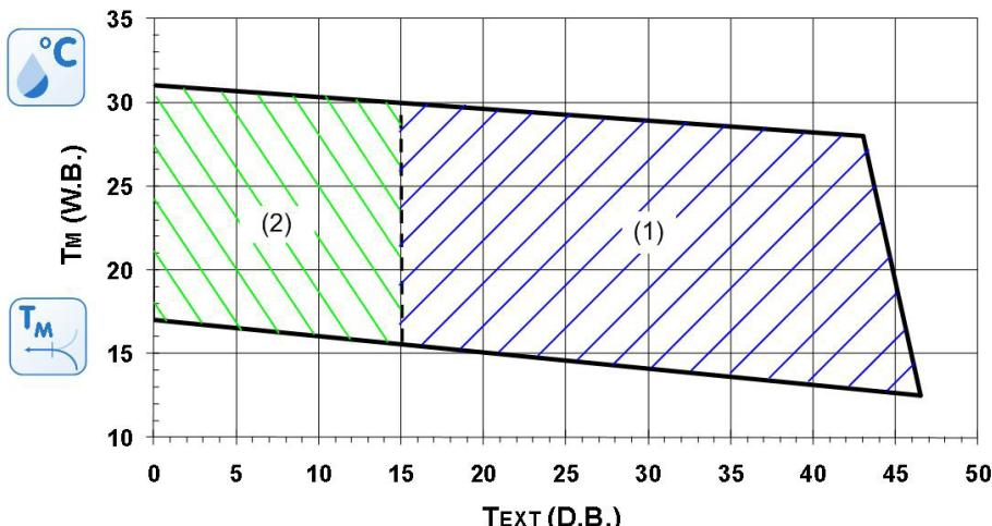
To verify the operating range of the operating units with percentages of fresh air, always calculate the T<sub>m</sub> mixing temperature at the internal heat exchanger input.
