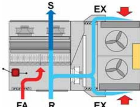
The room pressure control device is fitted as standard in the units with extraction and exhaust (Clivet reference code CCK and CKP)
