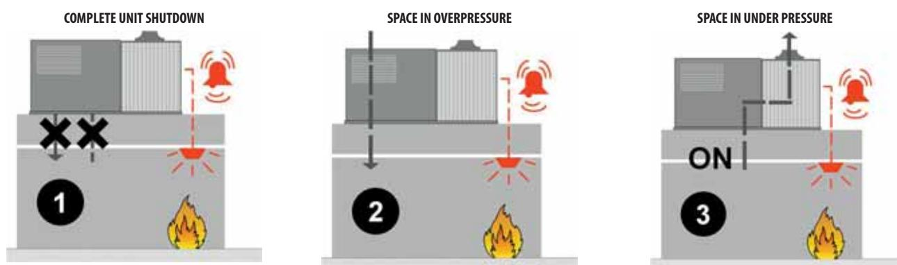
The unit is able to manage the signal coming from a fire detection system or fire control unit installed built-in, activating one of the logics illustrated, which can be set by parameters. In presence of alarm signal, the compressors are always switched off; moreover, the remote ON-OFF is disabled together with the switch on/off control from keypad. The unit is manually reset. Rooftop units cannot be used as fume extractor.
