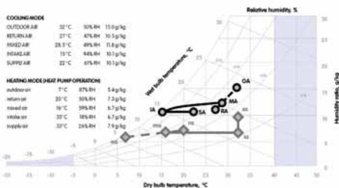
Treatment example at full load for CLIVETPack model CSNX-XHE2 20.4 in standard airflow. Outdoor airflow equal to 30% of that treated. Heating carried out with a heat pump. Unit complete with 'post-heating with hot gas' and 'vapour humidifier of 15 kg/h' options.
