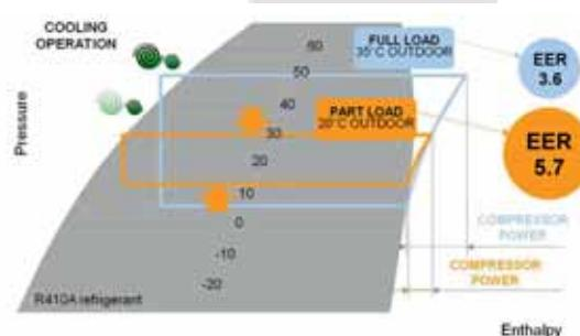
Example referred to CSNX-XHE2 33.4 in the all recirculation operation, according to EN 14511
