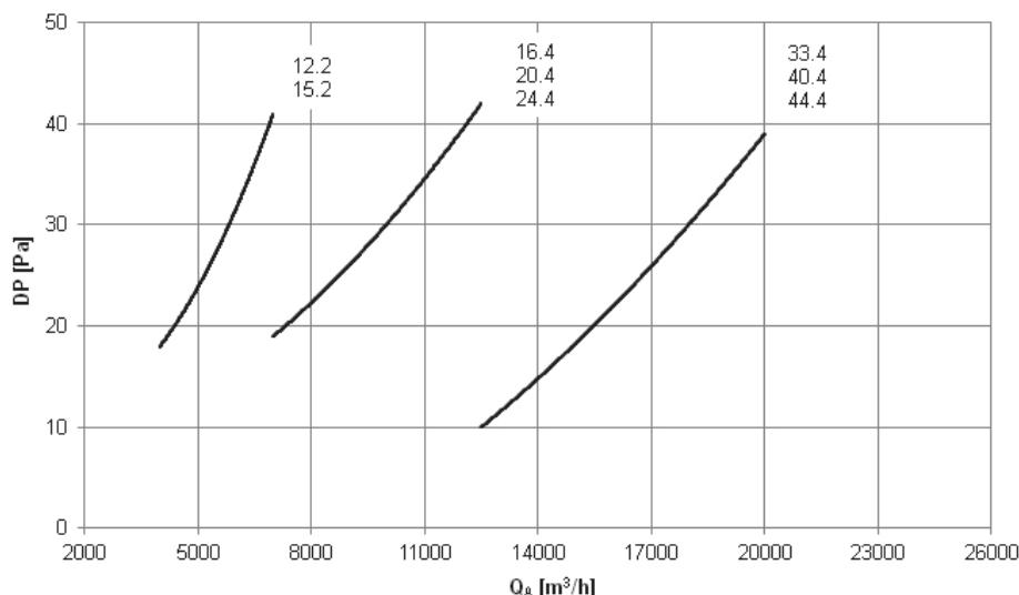
The air side pressure drops are relative to the medium air temperature of 20°C and are to be added to the pressure drops due to ducts, terminal devices and any other component that causes a drop in working discharge head.
