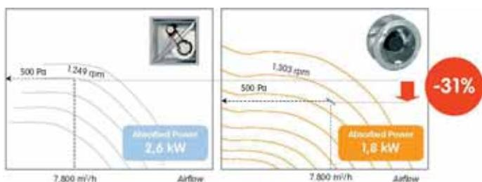
Electrical power absorbed by electric motor, data constructor - Example, referred to flow of 7,800 m³/h with 500 Pa external static pressure.
