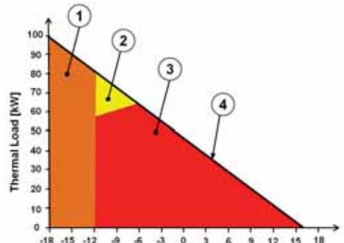
The load that needs to be met increases as the outdoor temperature drops.
