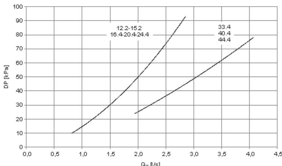
Pressure drops on the water side are calculated considering an average water temperature of 65°C
