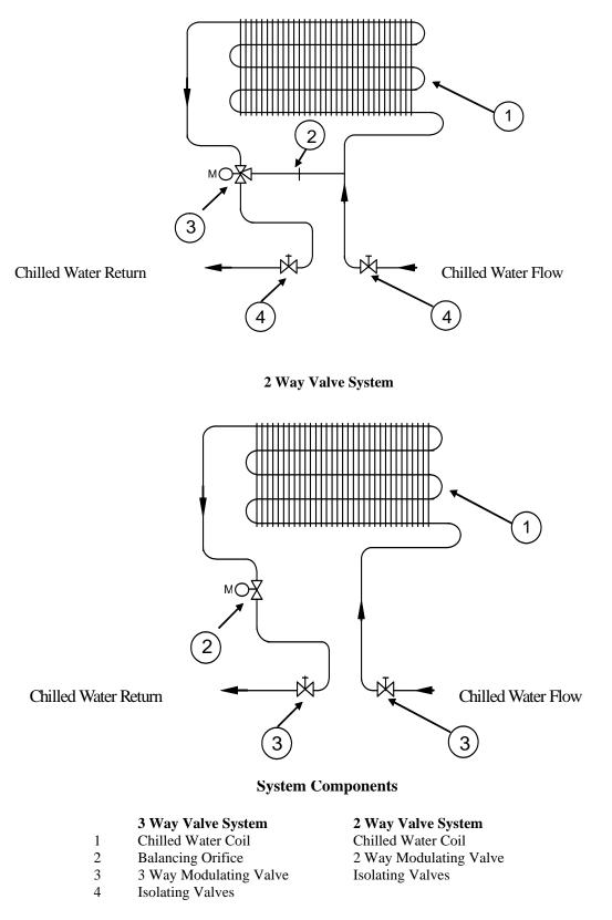
Note: Isolating valves are field fitted by others.
