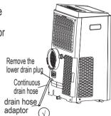
Direct the hose toward the drain, making sure that there are no kinks that will stop the warter flowing. Place the end of the hose into he drain and make sure the end of the hose is down to let the water flow smoothly. (See Figs with ◯ . Do never let it up. (See Figs with ◯ .). When the continuous drain hose is not used, ensure that the corresponding drain plug and knob are installed firmly to prevent leakage.
