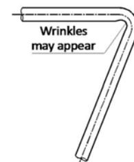
Figure 5.3: Pipe bending in excess of 90°
