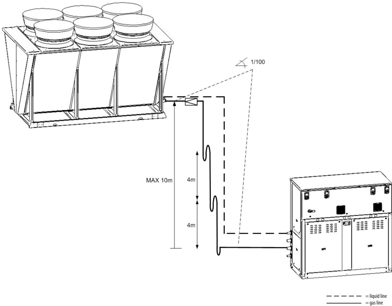
In the exemplifying connection diagram are represented only one supply piping (gas line) and one liquid piping. The number of lines must be doubled because the unit is equipped with a double refrigeration circuit.
