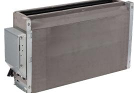
To add further ease during the installation phase, AURA presents the installer with the possibility of moving the water pipes to the right side of the unit even on site, simply by removing the heat exchange coil and turning it over. Consequently, the control panel on the unit can be moved from one side to the other as well.
