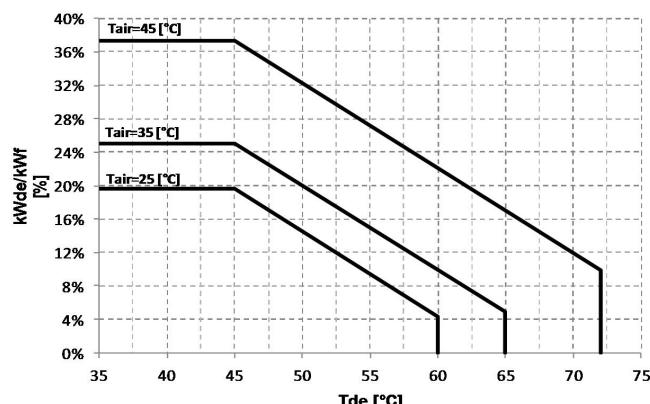
$kWde/kWf$  = Heat recovered/Cooling capacity [%]
