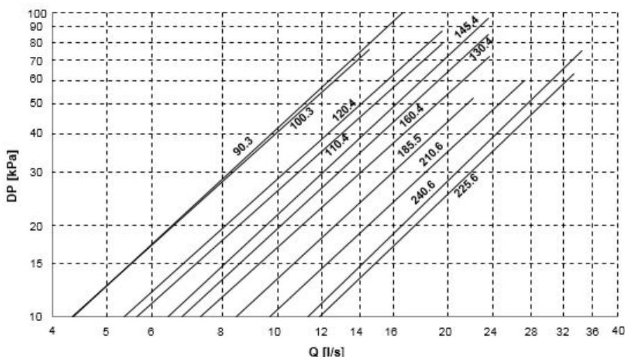
The pressure drops are calculated considering a water temperature of 7°C
