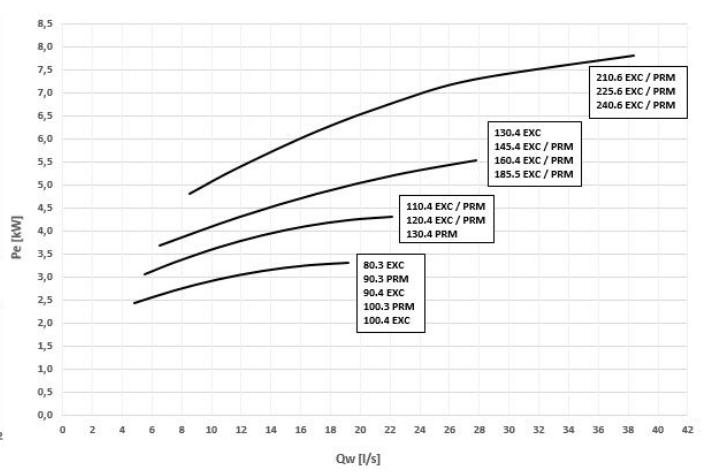
P<sub>e</sub> = Power input [kW]
