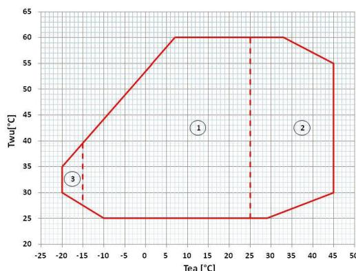
Twu [°C] = Water outlet temperature at the recovery side of the heat exchanger
