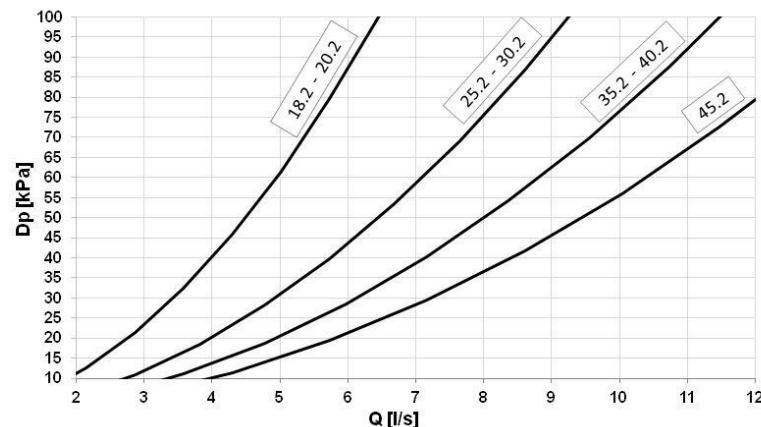
The pressure drops on the water side are calculated by considering an average water temperature at 7°C.
