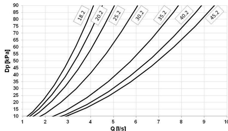
The pressure drops on the water side are calculated by considering an average water temperature at 7°C.
