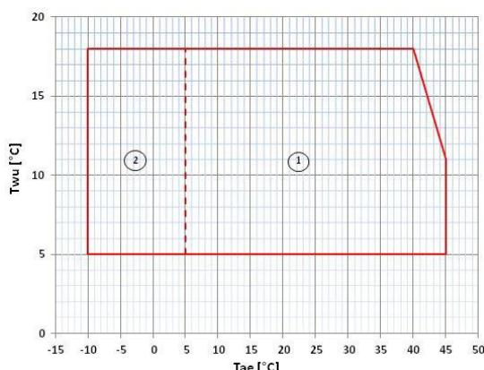
Twu [°C] = Internal exchanger outlet water temperature
