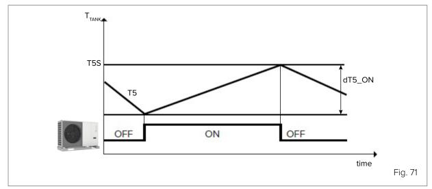
DHW is requested when T5S - T5  $\geq$  dT5\_ON
