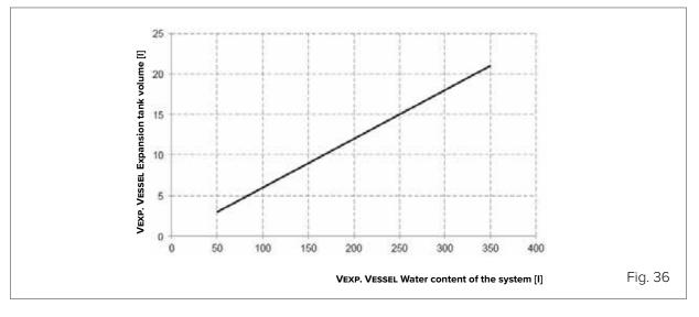
The volume of the additional expansion tank must be: VADDITIONAL = VEXP. VESSEL - 4.8 [I]
