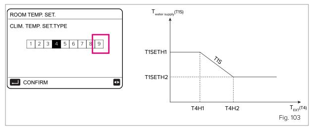
• 8 default curves for Cooling mode on systems with radiant distribution.
