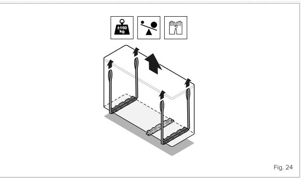
• Assemble the unit on the installation structure.
