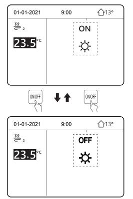
On the interface it is possible to switch on or off the unit for domestic hot water production.
