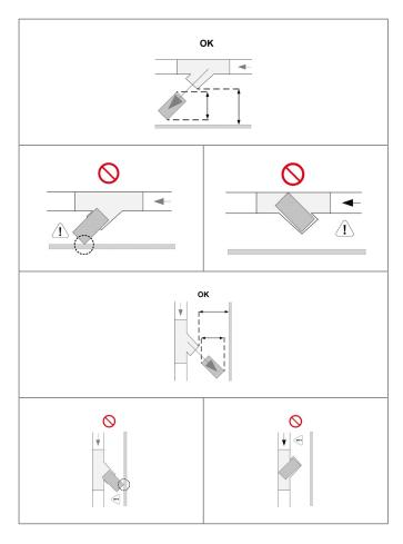
The filter must have an adequate mesh to prevent the entry of particles grater that:
