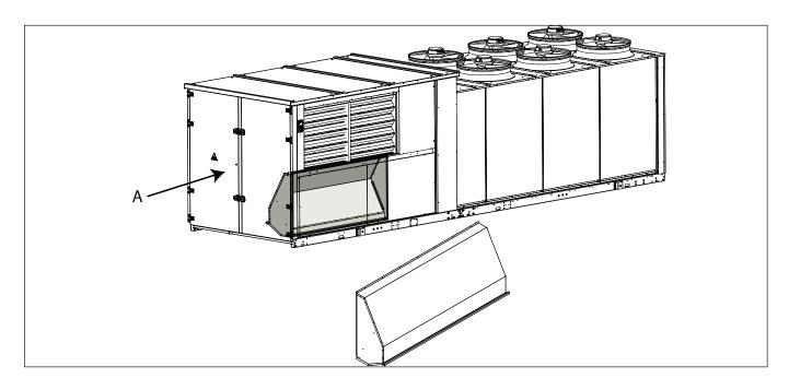
Open panel A, inside there is the hood and the fixing screws.
