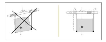
Align the barycenter to the lifting point
