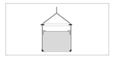
Lifting with spacer bar
